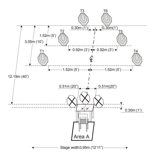
**SETUP NOTES:** Set paper targets to 1.52m (5 feet) at top of targets. X's for elbows placement are 6 inches (0.15m) right and left of centerline and 6 inches (0.15m) in from edge of table nearest competitor. Penalty targets are set so that the bases of the penalty targets are at table height. Area A is 4 feet (1.22m) by 4 feet (1.22m).
